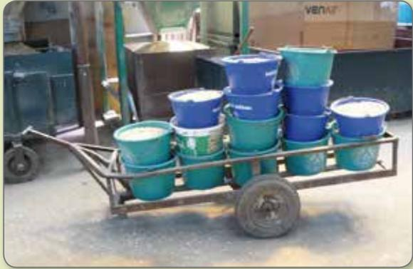
*With a barrow it is possible to carry multiple containers on one run. Use of this tool also permits a better distribution of the total load.*
