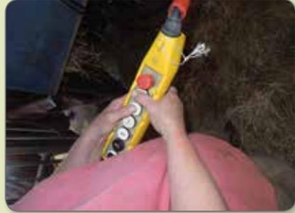
*Instead of manually distributing the food, a partly automatic cart can be used. This cart is mounted in a rail in the ceiling in the dairy stanchion barn. The worker just has to use the joystick to distribute the food. It is important to consider a distribution system that doesn't increase dust levels.*
