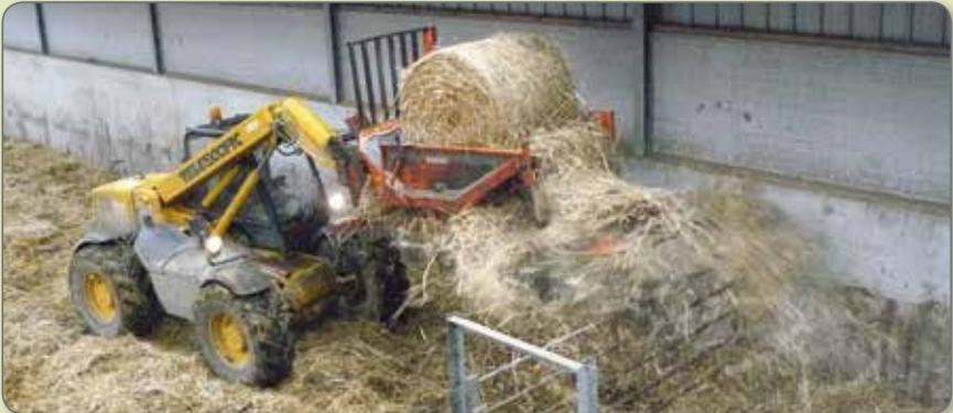
*The machine takes the ballot and puts it in the spreader with telescopic arm. No manual manipulation necessary.*
