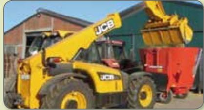
*By using a telescopic handler to take feed out of the silo, all manual handling can be avoided. The feed can then be placed in a feed mixer to be distributed.*
