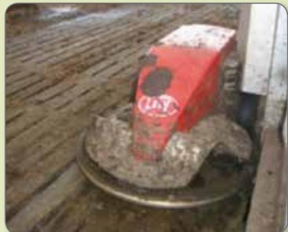
*Automatic manure robot is suitable in loose housing dairy barns with slatted floors. The robot reduces the heavy manual work task to a minimum.*
