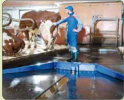
*This blade design is ideal for large volumes of manure, especially with straw bedding. In addition, the V formation gathers the manure cleanly and keeps pushing big loads forward, without spilling any manure back into the clean alley.*
