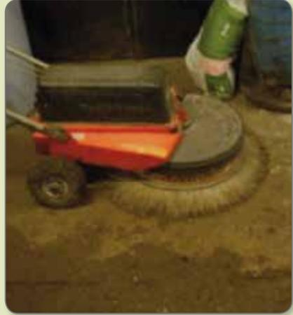
*Using a mechanical brush enables the adoption of a better posture to perform necessary cleaning. Moreover, uncomfortable muscular exertion can be avoided by using such mechanical aids. However, the user may be exposed to possibly harmful whole body or hand / arm vibration, so it would be advisable to take advantage of appropriate protection, such as an air suspended seat or wearing soft leather gloves. For more information see <http://www.hse.gov.uk/pubns/indg296.pdf>*
