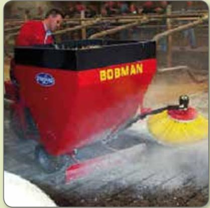
*Instead of manually distributing the bedding material, a small machine for bedding distribution can be used (left) or a machine where the distribution of bedding material is combined with cleaning/removal of small amounts of manure (right).*
