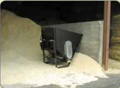
*A cart is mounted on a front loader or tractor and so the bedding material is distributed without any heavy work load.*
