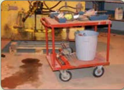
*The figure below shows a pneumatic tool for tightening (or removing) wheel nuts. The trolley carries the tool (which is heavy) plus ancillary equipment including a range of nut-spinner sizes and the hose, which must be connected to the compressor to use the tool.*
