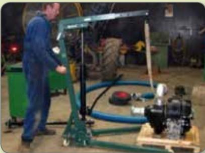
*Instead of carrying a heavy pump in the workplace, the farmer uses a manual crane.
