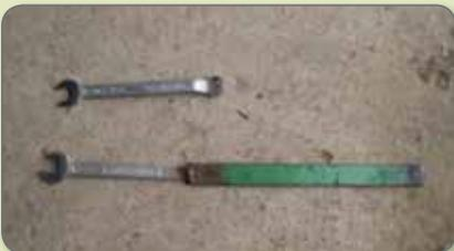
*This image shows a basic construction of a spanner. By extension, you are able to exert more torque but another benefit is to improve access to difficult places, such as when servicing agricultural machinery.*
