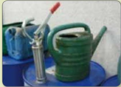
*Using a pump or a holder on the can, avoids the worker having to bend over when recharging his oil can.*
