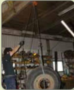
Using a tackle permits lifting and moving the tyre without carrying it. There are electric or manual tackles. It is always very important to check the strength of the supporting beam to avoid accidents. Once you start using it, the daily work becomes much easier.
