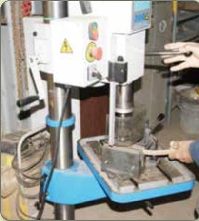
*A plastic shield prevents getting dust or other debris into your eyes. There is also the option to set the height of both the drill and vice so you can work in a correct posture, important when drilling several pieces.*
