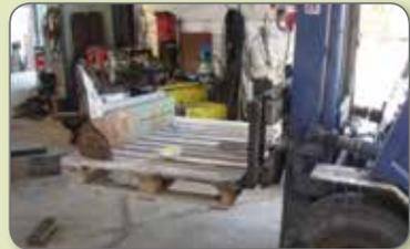
It may be possible to fix a pallet to the lifting forks of a fork-lift truck (FLT) to make a height-adjustable working surface.
