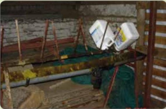
*The self-constructed rack, enables the farmer to leave the containers to drain themselves. The upturned containers are placed on the spikes and the remaining liquid falls into the channel below the spikes. All the waste can then drain out through the downpipe into a single collection point. This is similar to the guttering system for the roof of a house.*
