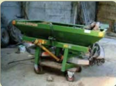
*A pallet with wheels can be used to store and to transport a machine. However, it is important to check whether the wheels can withstand heavy loads and use such pallets accordingly.*
