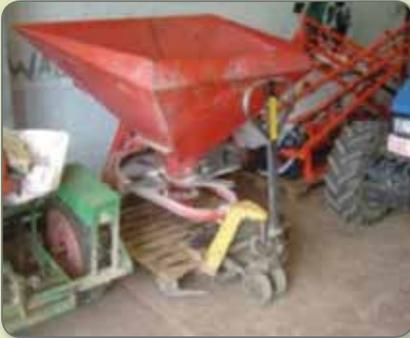
Using a pallet to store the machine and a pallet truck to move it not only helps to avoid unnecessary stresses and strains but also to avoid potential accidents. The machine is vertically stored, can easily be moved and coupled (the manual pallet truck can easily be lifted up to 20 m). The pallet truck must be pushed and not pulled.
