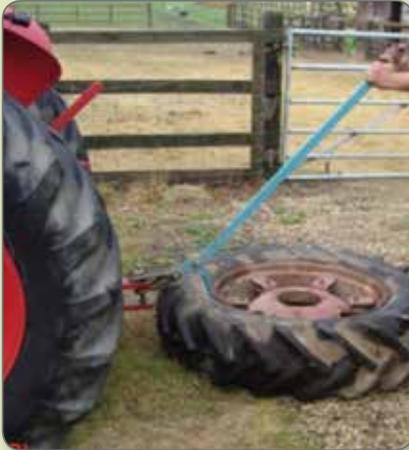
*An alternative approach has been designed by a young farmer which relies on using the mechanical advantage provided by a lever arrangement. It is simple to construct and much easier to use than the standard tool. It needs only one anchor point that, in the example shown, is provided by the tractor linkage assembly.*
