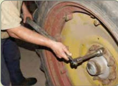
With the help of an ordinary iron pipe, the extra leverage makes it easier to apply more torque.
