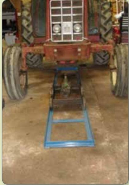
*For the separation of engine and gearbox, the front end can be moved from the rear end on a track, thereby avoiding lifting and ensuring the parts line up for re-assembly.*
