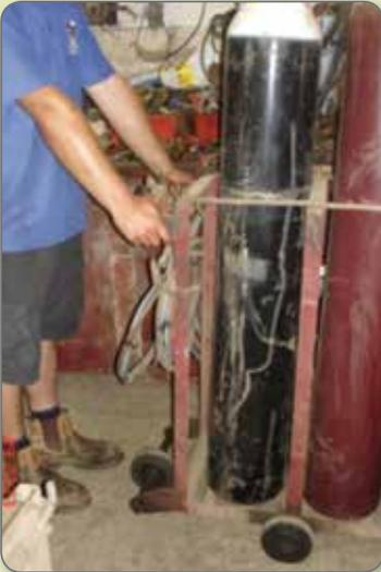
*It is easy to make, in almost any workshop, a more ergonomically designed trolley which is easier to move (handle height and weight of bottles balanced over axle) and allows easier access to the gas bottles for removal or replacement.*
