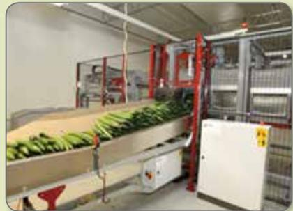
*The recently developed cucumber trolleys (see above), are unloaded at an automated working station, from which further sorting and packaging can start.*
