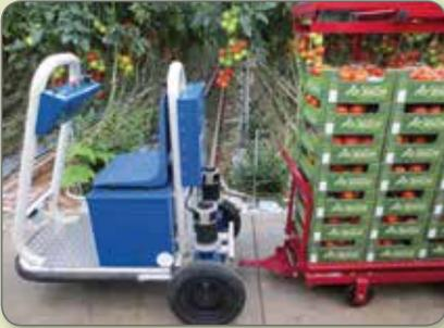
*By means of an electric truck for internal transport the trolleys can be transported automatically to the packaging area. The truck can be guided manually or fully automatically by following an induction wire which is built into the floor.*
