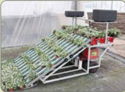
*Similar to the above example for lettuce, this device lifts the plant pots to enable the operator to work in a more comfortable (upright) posture. The device is powered by two batteries and can operate at a faster or slower speed.*
