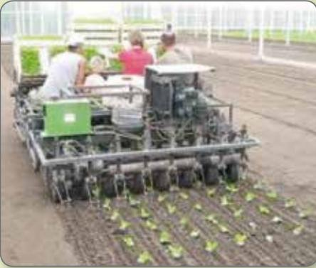
*A planting machine has a lot of advantages: cardiovascular load is significantly reduced, better posture of the back and higher productivity are the result. On the other hand, more reaching, repetition and prolonged sitting are present. The support to the lower back is minimal.*
