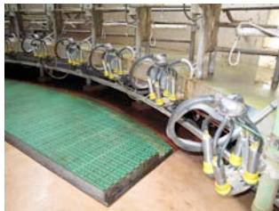
A floor in the milking parlour adjustable to the height of the milker
