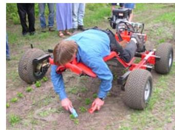
Various types of machinery to improve working postures of manual work at ground level. The lying posture may decrease the load on the lower back and pressure on the knees.
